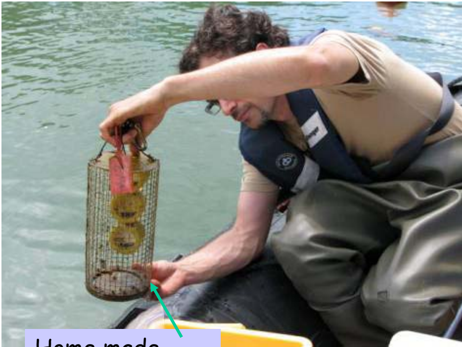
Home made exp. syst. for Chemcatcher
