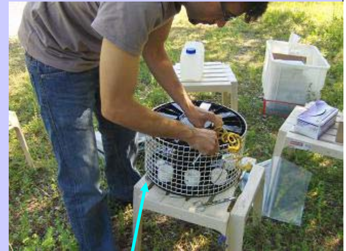
Home-made exp. syst. for chemcatcher
