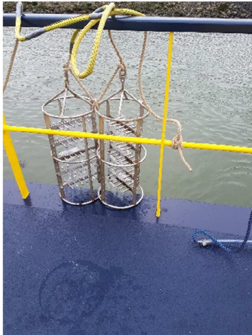
Exposure frames for silicone sheets
