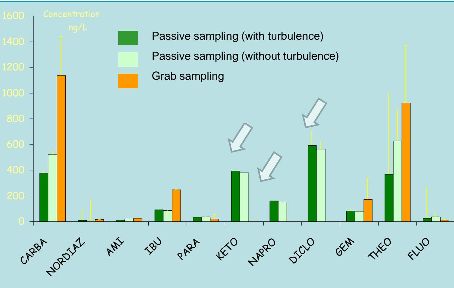
➤POCIS sampling allows to limit matrix effects (ketoprofene, naproxene and diclofenac)
